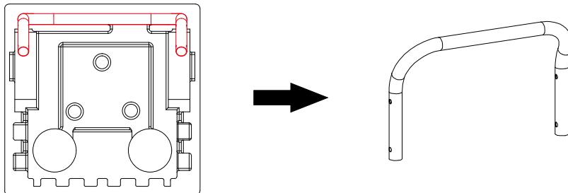
2) Install the handle as illustrated below, please note to align the holes on the handle with the holes on the dehumidifier. Use a screwdriver to tighten the screws until the handle is firmly attached to the dehumidifier.
